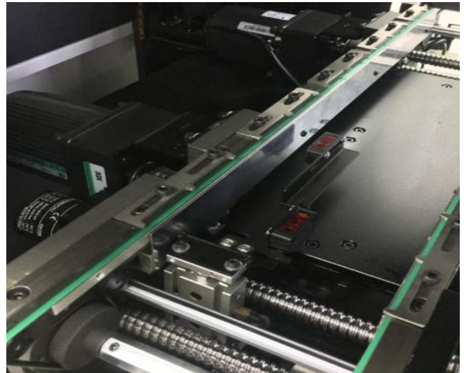
Integral casting structure, FPC compatible, PCB can be up to 1200*500mm.
