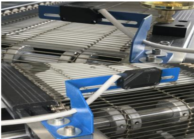
In and out board sensor monitoring, matching software board drop function detection, to prevent PCBA damage caused by reflow oven.
