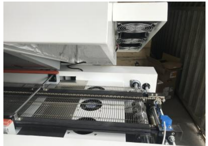
Under the condition of ensuring the length of the welding area, there are external fans at the bottom of the exhaust port and the outlet to cool the PCBA.
