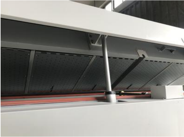
The use of electric struts facilitates the maintenance of the equipment and increases the safety of opening the furnace cover.
