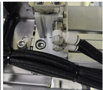
Additional protection of all access lines
