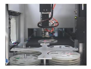
Load the materials on the loading truck, push the trolley to the corresponding position, close the warehouse door, and start the program
