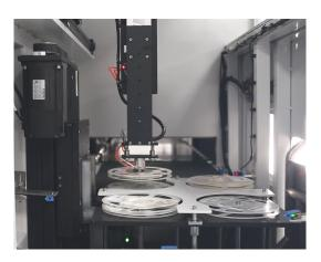
After the ordering is completed, the material is shipped out of the warehouse. The camera automatically takes a picture and locates it. The gripper sticks the new barcode to the corresponding position and takes a picture again to identify and locate it. The gripper puts the material tray into the material cart to complete the ordering of materials.
