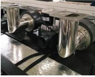
I.C.T cooling system is more reasonable, water cooling and air cooling can be replaced at any time, and nitrogen in the cooling zone can be monitored
